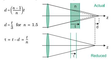
The **reduced thickness**  $\tau$  gives the air-equivalent thickness of the glass plate. A **reduced diagram** shows the amount of air path needed to fit the plate in the system, and no refraction is shown at the faces of the plate. A **reduced tunnel diagram**
