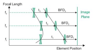
As the separation approaches the sum of the element focal lengths  $(f_1+f_2)$ , the system becomes afocal  $(f \to \infty)$ . The zoom range of the analogous **telephoto zoom** is limited by its BFD as the rear element can run into the image plane when the element separation approaches  $f_1$ .
