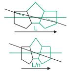
shortens the length of a tunnel diagram by 1/n to show the airequivalent length of the prism. Reduced diagrams can be placed directly onto system layout drawings to determine the required prism aperture sizes for a given FOV. Note that the OPL increases greatly when a prism or glass plate is inserted.
