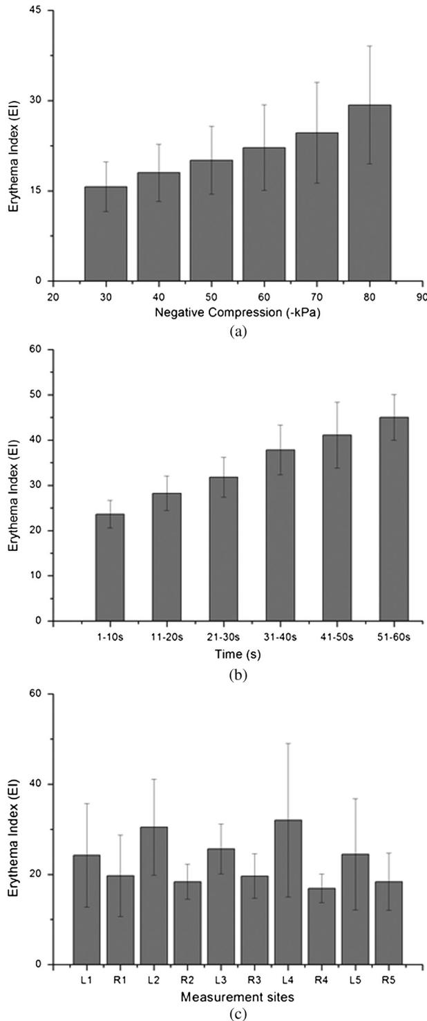
**Fig. 3** Erythema index (EI) variation as a function of (a) negative compression, (b) time at a constant negative compression of  $-80$  kPa, and (c) for 10 different measurement sites at a constant negative compression of  $-80$  kPa.
