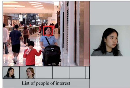
Fig. 9 (a) FD is well developed and commercialized in most modern cameras by different brands. This example of FD is from Google. (b) An example of multiple cameras adopted for surveillance in a long corridor for monitoring passengers. (c) An aided target recognition system for inspectors to take a closer second look at the specific passenger who has the same (or similar) pose of mug shots in the system. The two mug-shots are selected from MIT face databases. 33
