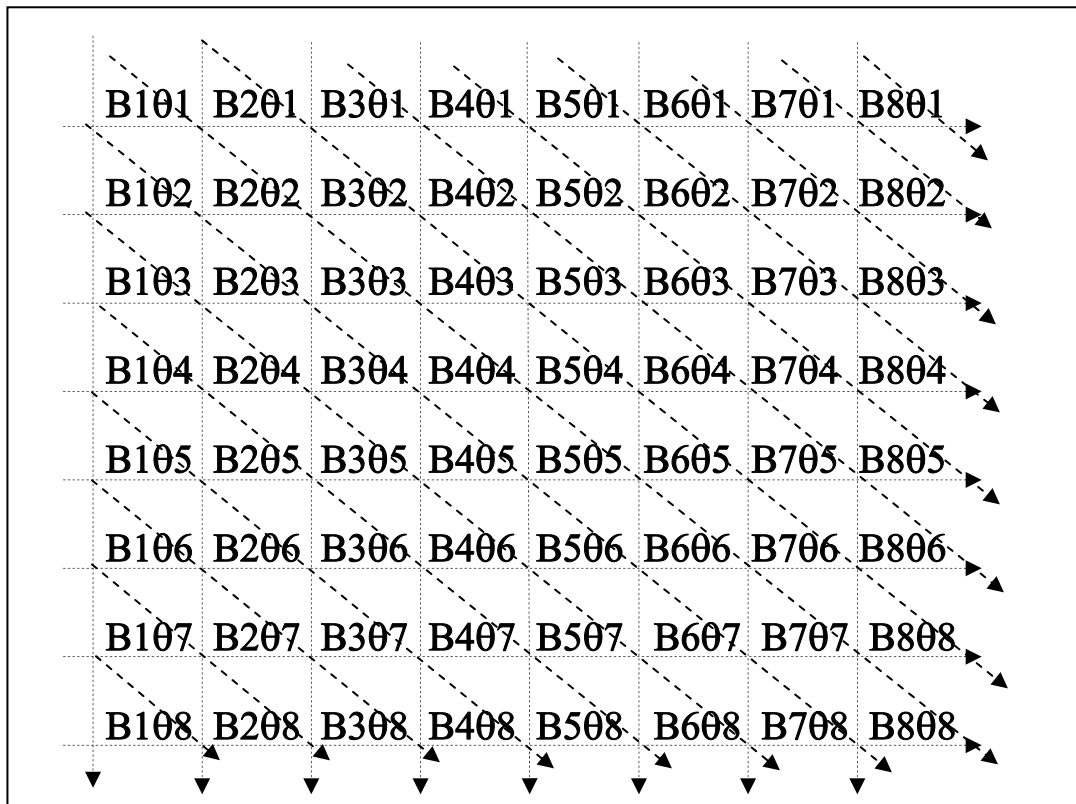
Fig.2 Schematic representation of a CW EPR two dimensional projection matrix. Let 8 projections be taken in 8 equally spaced orientations in a plane and let each projection be represented in 8 field steps, for simplicity. In the conventional slow sweep CW imaging the projections are gathered sequentially along the horizontal arrows each with constant angle \theta_n and 8 field positions B1 to B8. In the case of Ohno et al. and Deng et al., the field is stepped in 8 steps and at each field position, the gradients completes one full rotation ( \theta_1 to \theta_8 ), corresponding to the vertical arrows. After collecting the data, it is to be reshuffled by taking the first point in each of the field steps as the first projection, and the second in each field step constituting the second projection, and so on.
