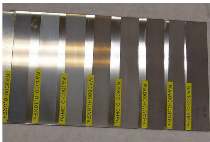
Fig. 4. An example of the experiment to determine the process condition of the sandblasting. Fluorescent lights reflecting on the surface can be observed.
