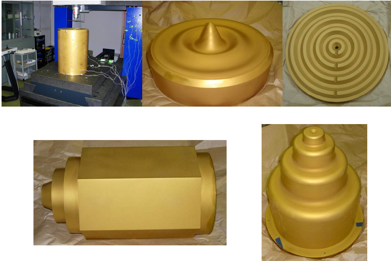
Fig. 7. Gauges for checking the practical performance of non-contact CMMs.
