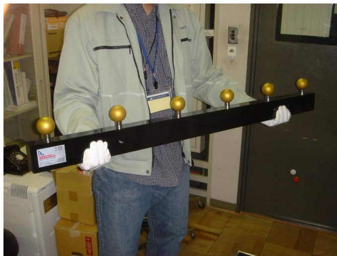
Fig. 6. A ball array made by the consortium for assessing the error of indication for length measurement.
