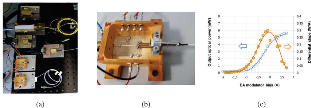
Figure 9. RF photonic transmitters for multi-RF photonic frequency conversion
