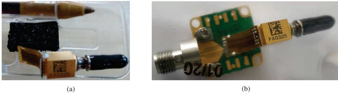
Figure 1. (a) EML sample to be evaluated, (b) EML mounted onto a PCB for testing
