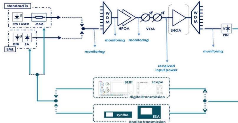
Figure 11. Test set-up for FSO transmission experiments
