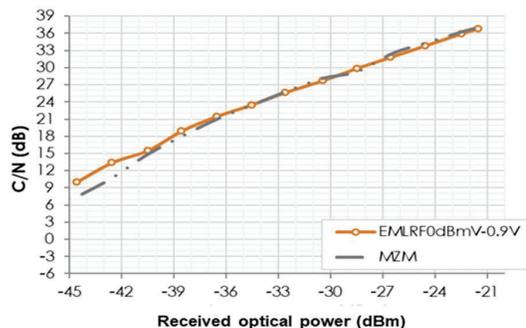
Figure 13. Analog C/N measurements for FSO transmission of RF signals at 20 GHz ; comparison between EML and MZM
