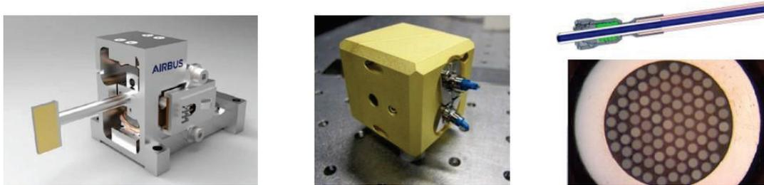
Figure 5 Left) ICC HW status decorrelation mechanism. Middle) Integrating sphere. Right) Transfer fiber bundle.
