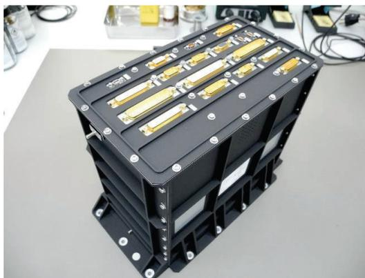
Figure 8 Merlin instrument control unit – PFM.
