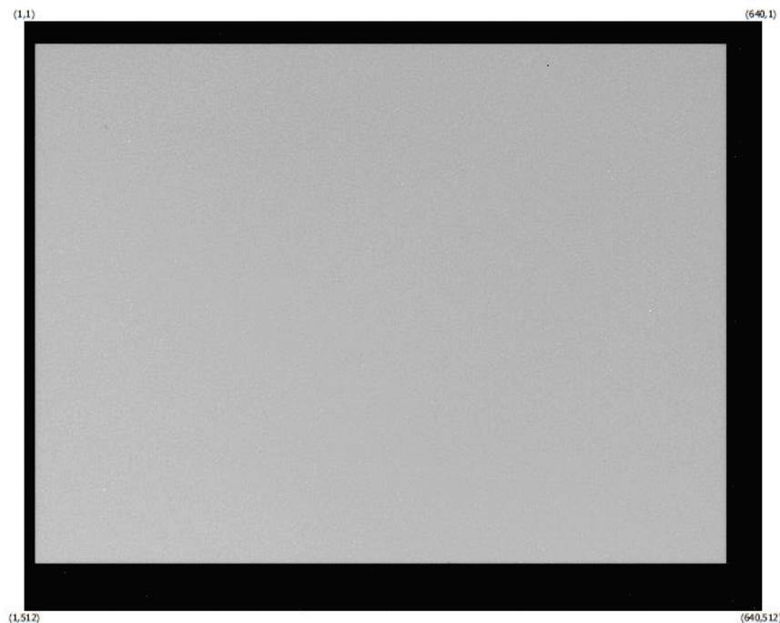
Figure 5: A plot of the output of a masked long wave device (640 x 512 24 $\mu$ m) which consists of a greyscale (lighter for higher signal and darker for lower signal). Masked pixels can be seen as a dark border, 10 columns to the left, 30 to the right, 20 rows at the top and 40 at the bottom. The array in question is imaging a flat field at 40°C.
