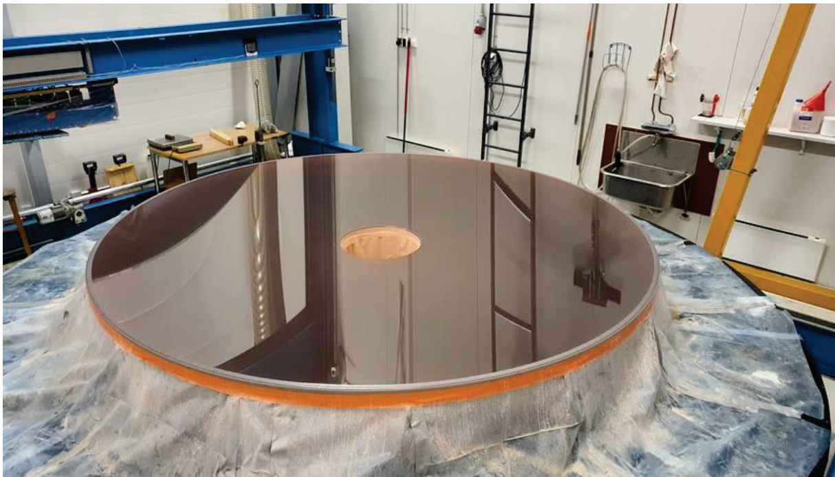
Figure 12. 2.6 m UV collimator at OPTEON Oy after polishing.
