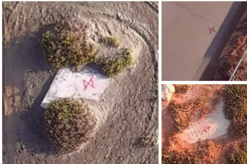
Figure 2 Ground control points (GCPs)
