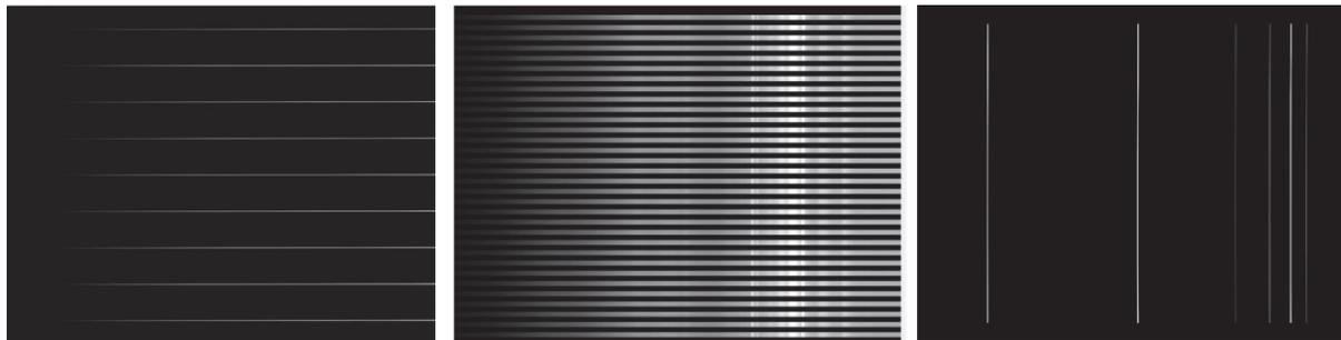
Figure 16. Three possible combinations of object targets and light sources used during the alignment at the USA focal plane. From left to right: Eq99 with pinholes, Eq99 with focusing pattern, flat field illumination with UV-VIS lasers.
