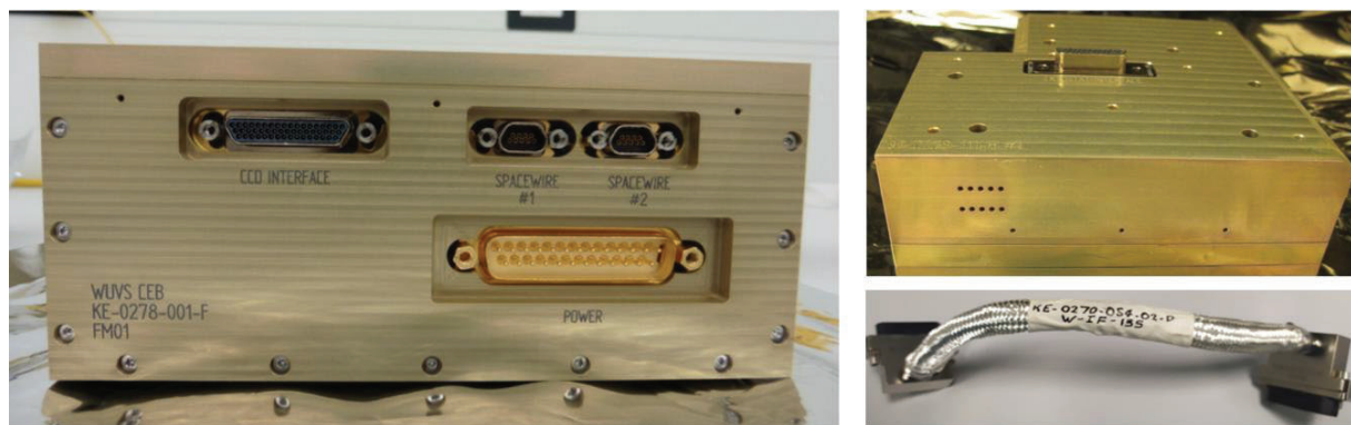
Figure 10. Flight models of the Camera Electronic Box (CEB), Interconnection module (ICM) and analog video cable.
