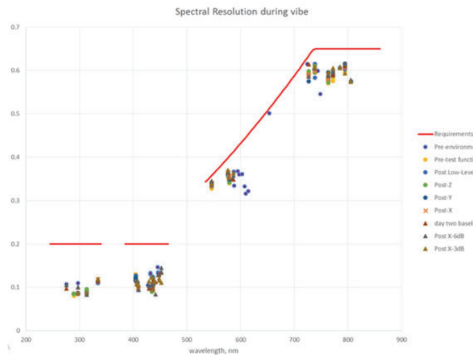
Figure 24: BU spectrometers spectral resolution over the 245 - 853 nm spectral range, and at different steps of the qualification tests. Credit: SuperCam.
