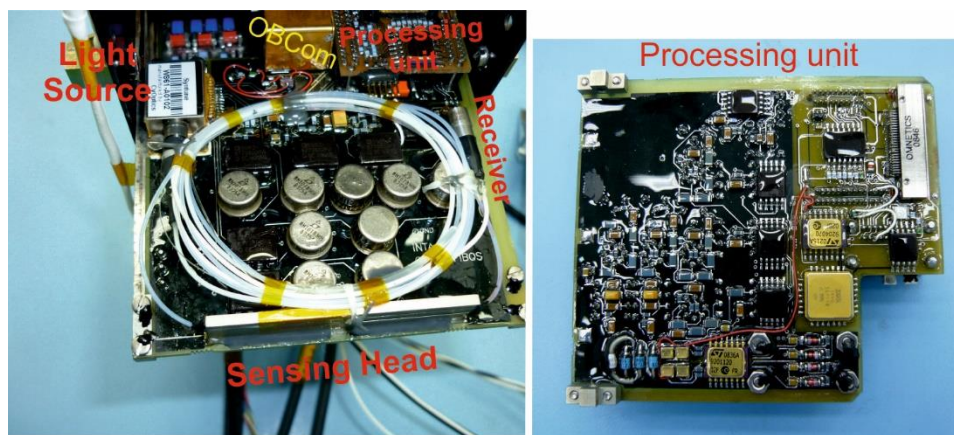
Figure 2. Left: FIBOS top view – FIBOS units and OBCom module. Right: FIBOS bottom view - Processing unit electronics
