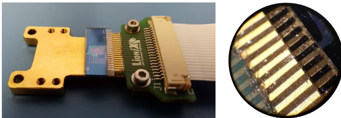
Figure 9: Picture of submount with LC switching chip (left) and detail of electrode connection (right).
