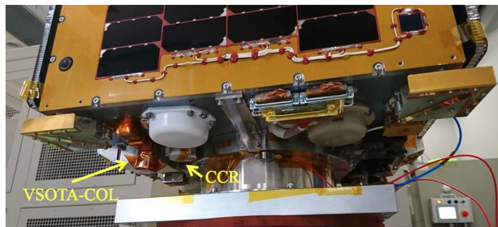
Figure 5. VSOTA-COL and CCR shown on the flight model of RISESAT
