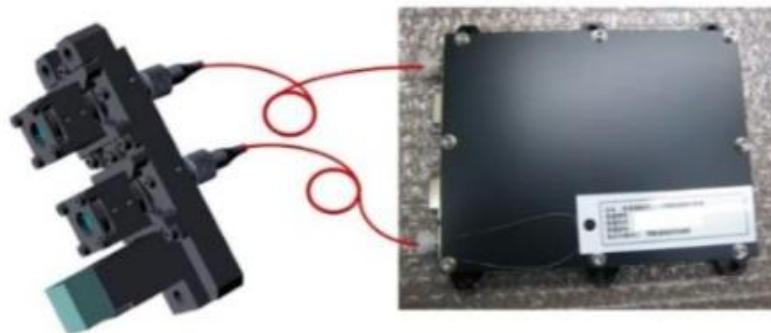
Figure 2. VSOTA pre-manufacture illustration of VSOTA-COL and flight model of VSOTA-E
