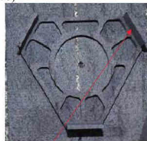
Blades machined separately and assembled at greenbody level
