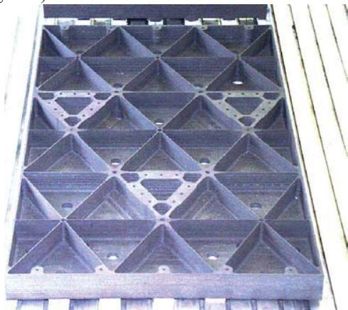
Figure 3 view of a 1 meter milled panel
