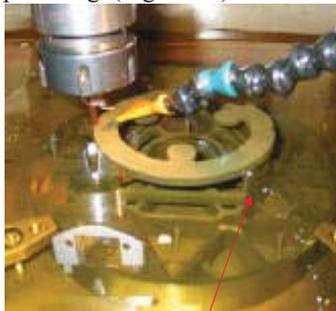
Filtering blades finished by EDM
