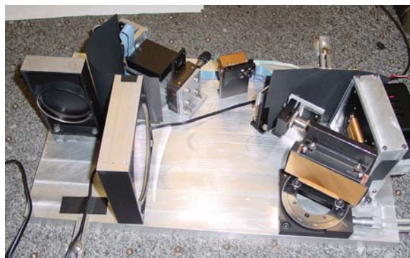
Fig. 5 The layout of the echelle-AOTF spectrometer bread board.
