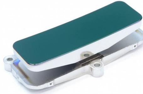
Fig. 3: Schematic overview of the black mirror design (left) and a picture of a mirror with the black mirror coating (right)
