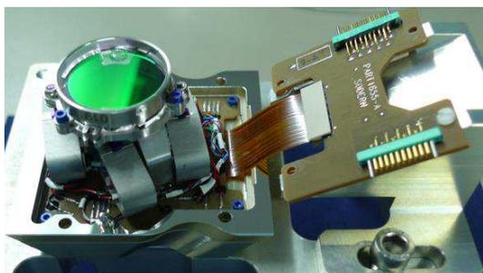
Fig. 1. Pointing mechanism – part of BSMFE
