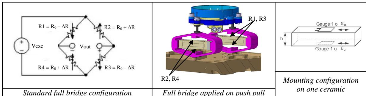
**Fig. 7.** Selected Full bridge configuration and its application on the push pull piezomechanism
