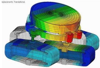
**Fig. 5.** FEM simulations result: Calculated maximum displacements during RX actuation
