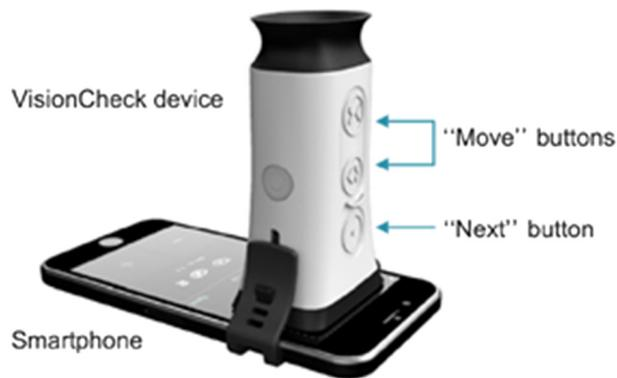
**Fig. 2** EyeQue VisionCheck device (shown as attached to a smartphone).
