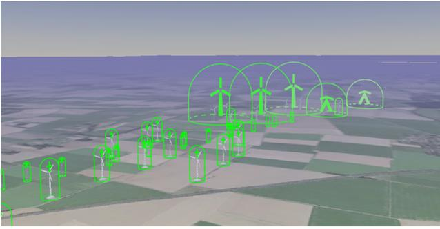
**Fig. 11** HMD obstacle representation with glass domes.
