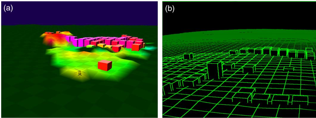
**Fig. 1** “Manhattan” obstacle symbology for degraded visual environment: (a) head down, (b) HMD.
