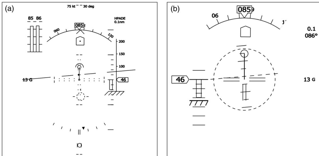
Fig. 7 (a) BOSS and (b) DEVILA landing displays.
