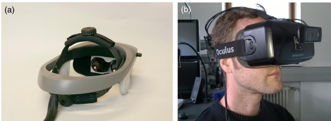
**Fig. 3** VR helmet-mounted display systems: (a) NVIS cybergoggle nVisor SX, (b) Oculus Rift DK2.
