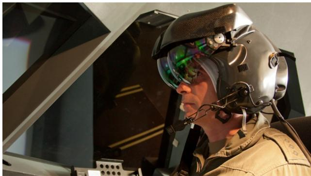
**Fig. 2** Wide-field-of-view helmet-mounted display system.
