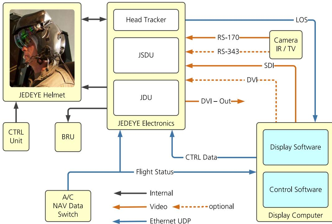
Fig. 4 Functional integration of HMD system into environment.
