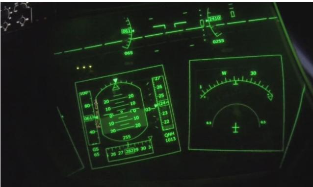
**Fig. 14** Virtual flight deck instruments as seen through the HMD.
