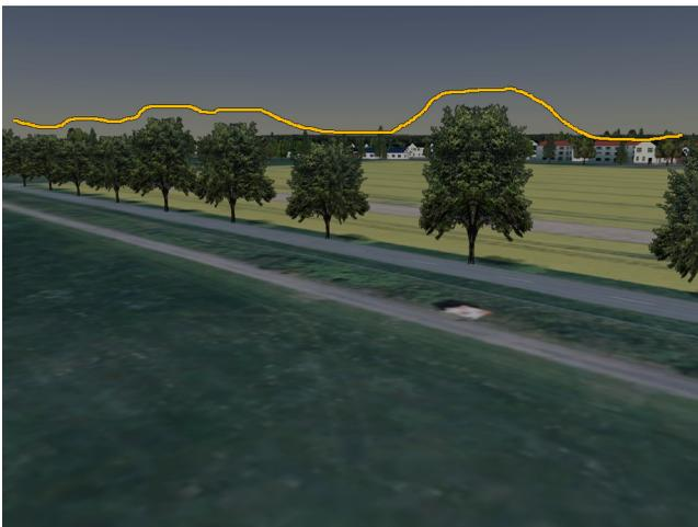
**Fig. 13** Concept of a safety line: the amber line represents a safe escape elevation angle.
