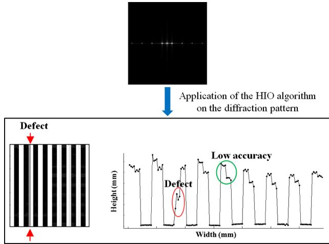
**Fig. 4** HIO algorithm enables to retrieve the global shape of the mask pattern, but accuracy is too low to determine precisely the depth of the defect.
