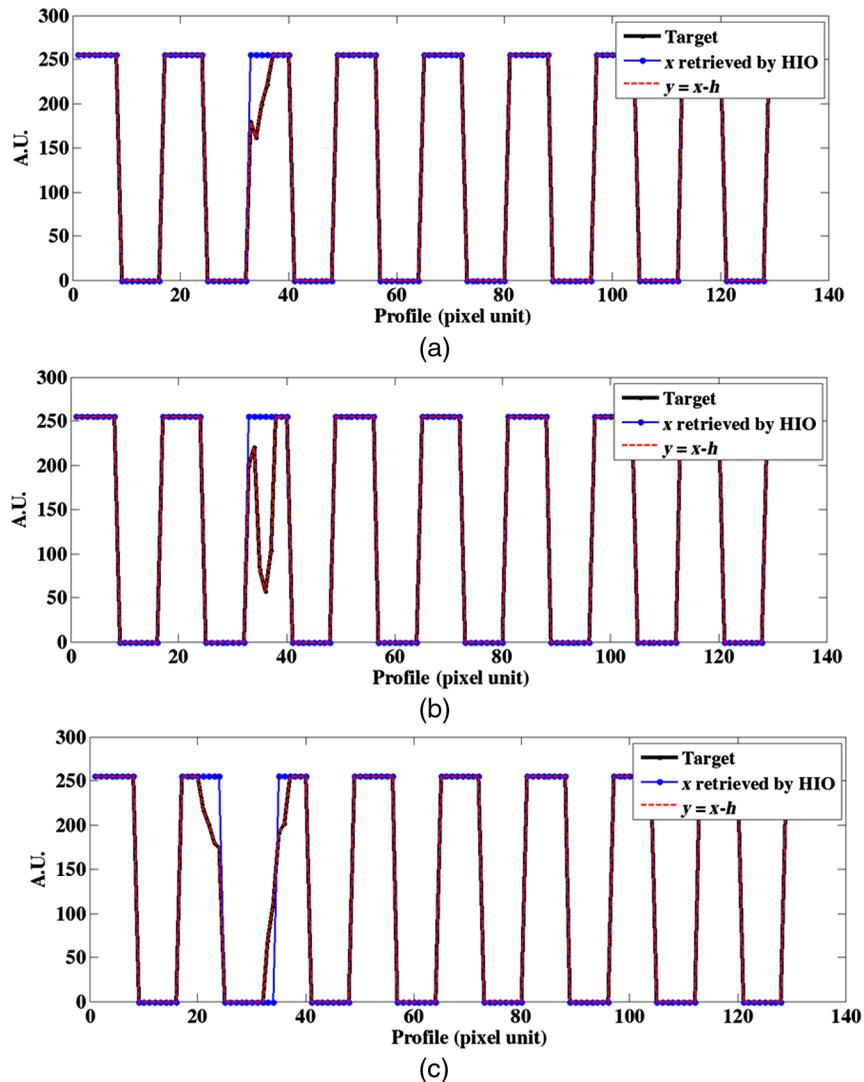
**Fig. 8** Example of defect characterization with our proposed method. Several cases were tested including (a) small defect, (b) defect with both positive and negative components, and (c) defects on two different stripes.
