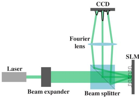
**Fig. 9** Experimental setup. Different mask profiles are displayed on the SLM and the patterns diffracted are acquired with a CCD camera.
