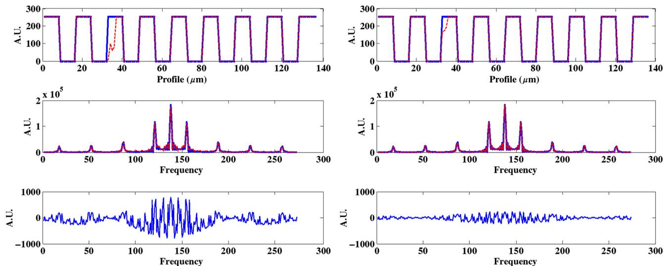
Fig. 2 Effect of defects on the diffraction pattern. The first line represents the mask profile with (red) and without defect (blue), the second line shows the amplitude of the diffraction pattern in one dimension, and the third line represents the subtraction between the two diffraction profiles.
