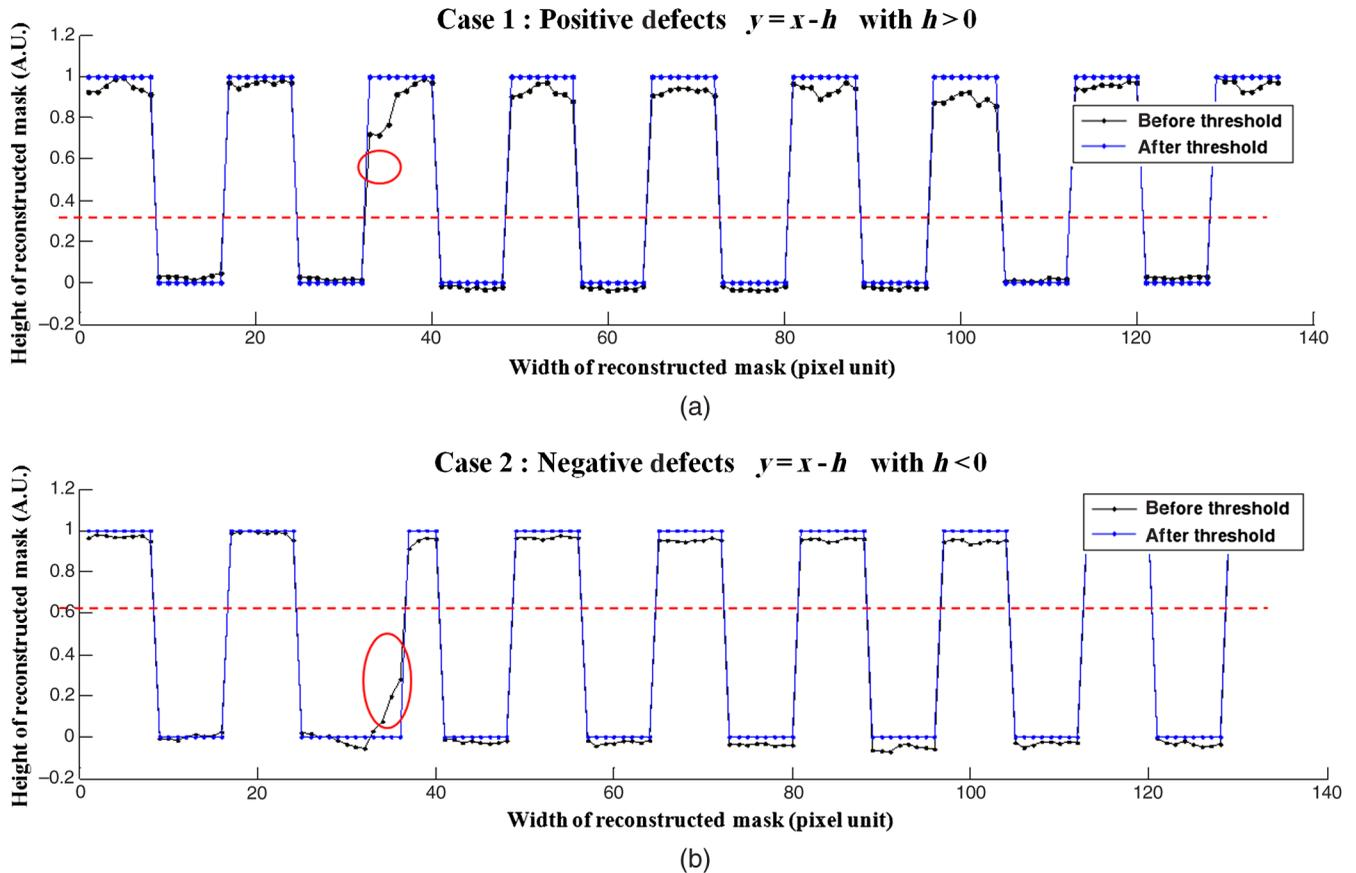
Fig. 7 After application of the HIO algorithm, a threshold filter is applied to obtain the reference profile. Since the pattern is not defect free, two cases may happen depending if the defect is (a) above or (b) under the threshold value (red line).
