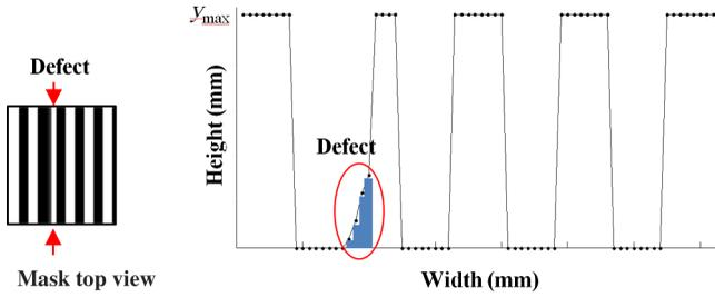
Fig. 1 Top view and profile of the type of mask considered.
