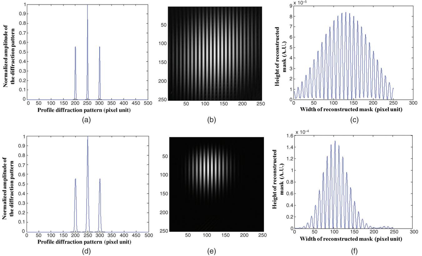
**Fig. 5** Masks (b) and (e) are recovered from diffraction patterns with (a) narrow and (b) medium spots width, respectively. Only a one-dimensional (1-D) profile of the diffraction patterns is illustrated. The profiles (c) and (f) are 1-D illustration of the mask (b) and (e), respectively.
