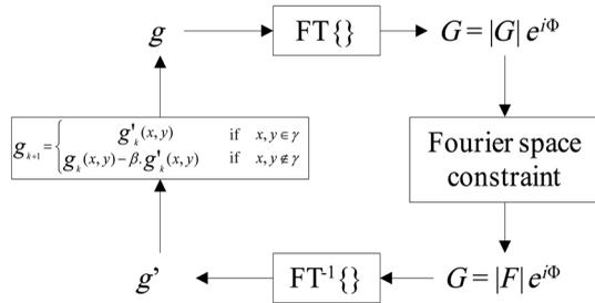
**Fig. 3** Principle of the HIO algorithm. The support of the image is noted  $\gamma$ , and  $|F|$  is the known amplitude of the Fourier pattern.
