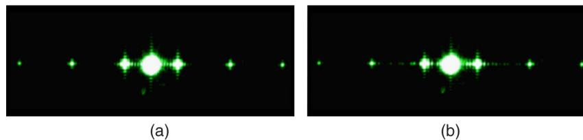
**Fig. 10** Diffraction pattern from (a) a defect-free mask and (b) a mask presenting a defect.
