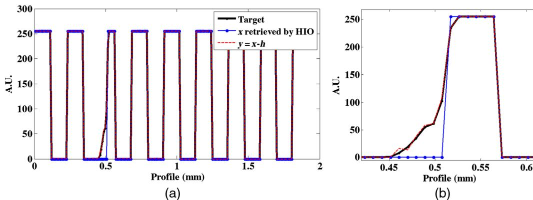
**Fig. 11** Example of the total profile reconstruction from the diffraction pattern captured by CCD (a), with a zoom at the defect location (b).
