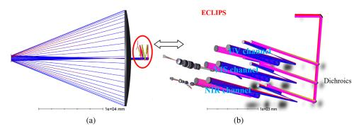
**Fig. 2** (a) On-axis 15-m LUVOIR TMA telescope and ECLIPS position relative to the telescope. (b) ECLIPS coronagraph channels and their modules. The three channels are split by dichroic beam-splitters in order to obtain the images from different channels simultaneously.
