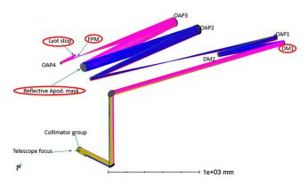
**Fig. 3** ECLIPS coronagraph optical layout. The labels with red circles are the four key coronagraph elements: DM1 and coronagraph masks. The figure shows that they are located at the four critical planes, as described in Sec. 2.
