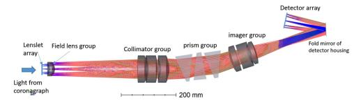
**Fig. 7** Optical IFS design. The field lens is used to control the chief rays to reduce the diameter of the collimator group. The compound prisms are to provide the required spectral resolving power. Meanwhile, the material selection of three prisms is for making the spectral resolving power as flat as possible in the defined wavelength range.
