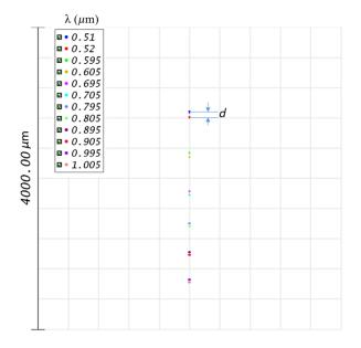
**Fig. 8** The spot diagram at detector array for full wavelength range at the central FoV. The box on the upper-left corner indicates the wavelength in microns of each spot. The wavelength separation of each pair of spots is 10 nm. The physical separation d on detector array is calculated by Zemax ray trace.
