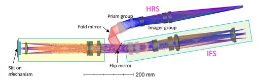
Fig. 12 NIR HRS design. A flip in and out mirror with a mechanism is used to switch between the NIR IFS and the HRS. The additional fold mirror in the HRS channel is just used for packaging.
