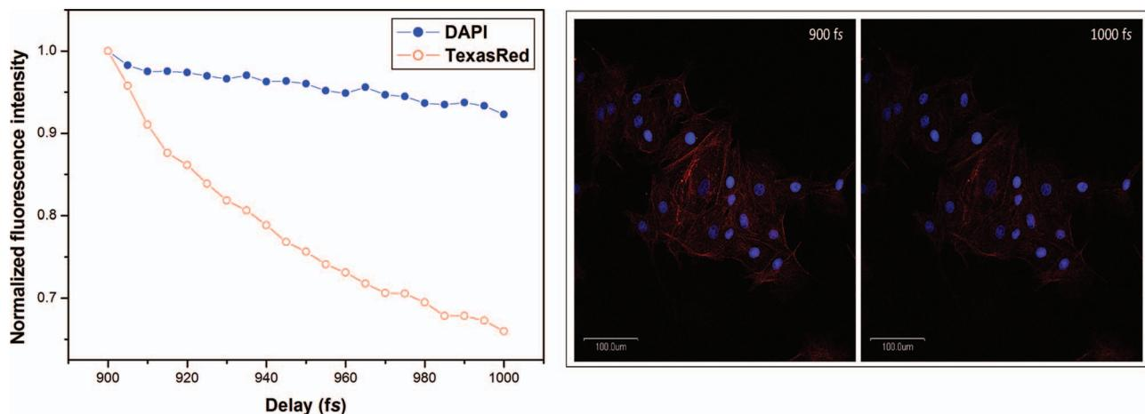
**Fig. 2** Selective two-photon fluorescence suppression for Texas Red (open circle) compared with DAPI (solid circle) under pulse-pair excitation.
