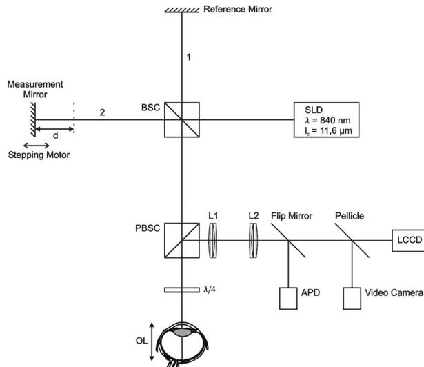
**Fig. 2** Optical setup: SLD, super luminescent diode; BSC, beamsplitter cube; PBSC, polarizing beamsplitter cube; APD, avalanche photo diode; and LCCD, linear CCD array. Depth ranging is provided by a scanning mirror.
