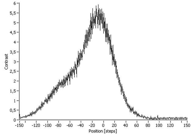
**Fig. 5** Fringe contrast of an artificial eye plotted against the position of the measurement mirror.
