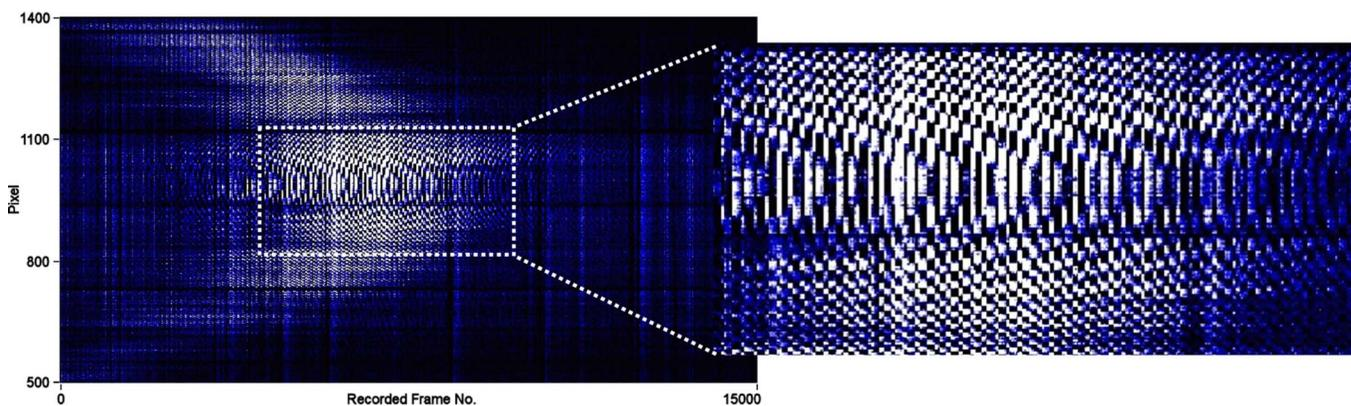
**Fig. 4** Synthetic interferogram recorded from an artificial eye while moving the measurement mirror over a range of  $75 \mu\text{m}$  around the optical length of the sample.
