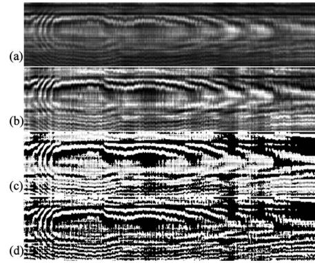
**Fig. 7** Steps of image enhancement demonstrated on a synthetic interferogram recorded *in vivo* over one pulse period.
