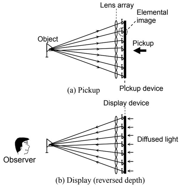
Fig. 1: Basic principle behind integral method
