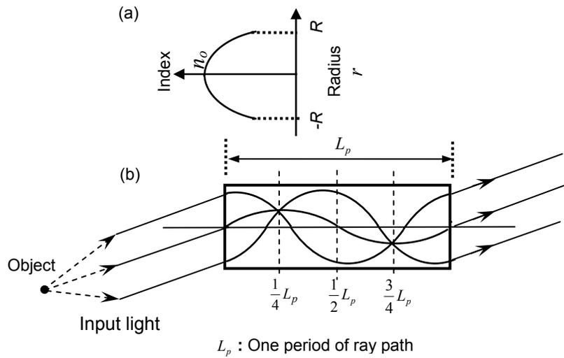
Fig.3: (a) Refractive index of radial GRIN lens.
