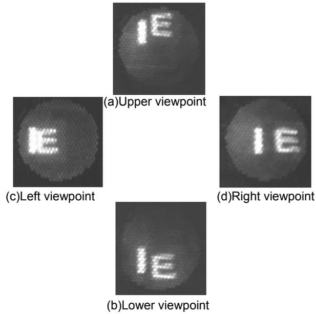
Fig. 6: Photographs of images formed by the optical viewer. Four viewpoints are all away from center axis of exit plane by approx. 9 deg.
