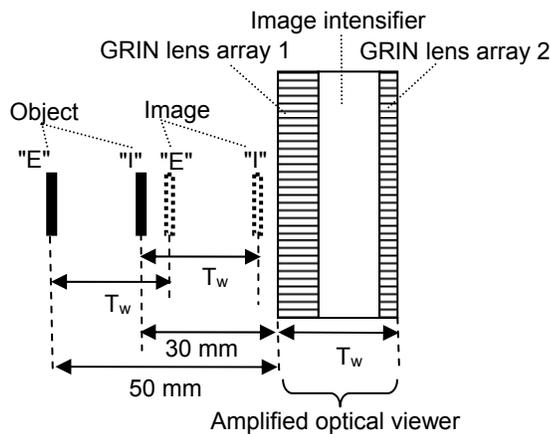
Fig. 5: Experiment using amplified optical viewer (side view). Objects I and E are letters both with 32-point font. I is 30 mm from array 1 and E is 50 mm from same array. Center of both letters is offset 6 mm horizontally. Both images are separated from two object positions by  $T_w$  (45.5 mm), i.e., thickness of amplified optical viewer.
