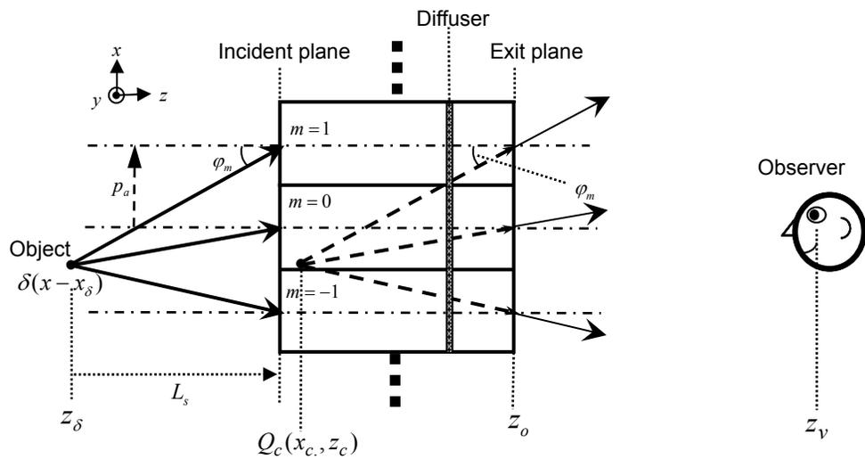
Fig. 4: Geometric view of optical viewer
