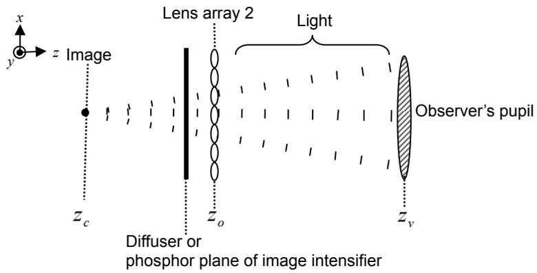
Fig. 7: Reproduced image behind exit plane of optical viewer
