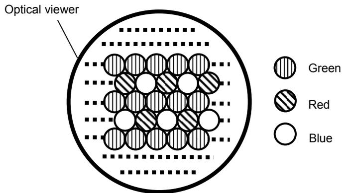
Fig.10: An example of the color filter arrays on the incident plane and the exit plane with the same structure.
