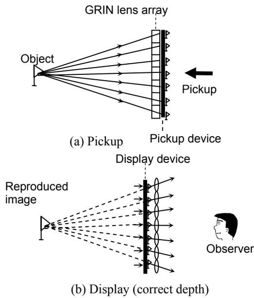
Fig. 2: Integral method with orthoscopic image
