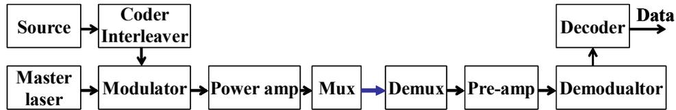
Figure 7. Communication subsystem
