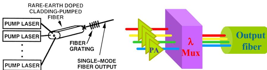
Figure 8. Double-clad erbium amplifier and multiplexer.
