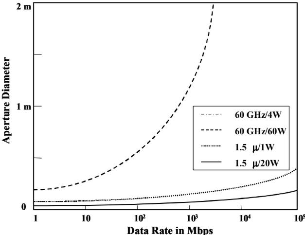
Figure 3. Crosslink aperture size for RF and optical links with geosynchronous range.
