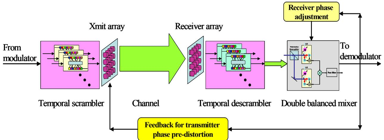
Figure 20. Transmission system block diagram; not all subsystems shown (including: modulator/demodulator, coder/decoder, frequency shifters, optical amplifiers etc.).
