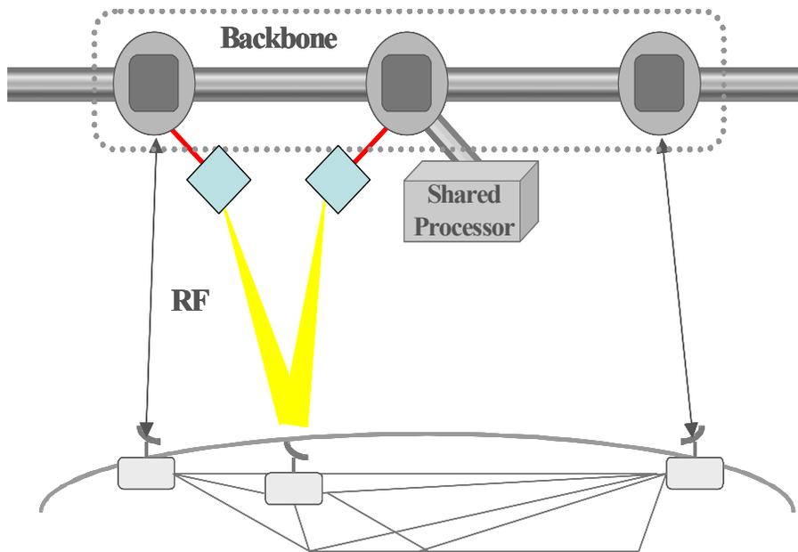
Figure 24. Multi-platform distributed space communications
