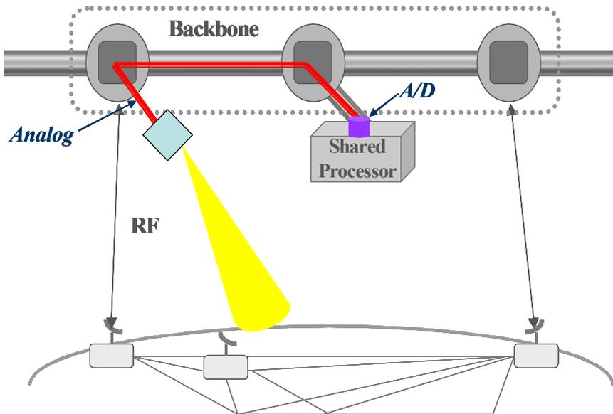
Figure 23. Reconfigurable and upgradeable RF satellite access network.
