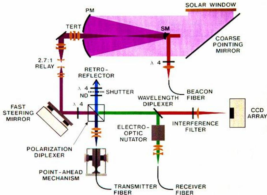
Figure 6. Optical subsystem.
