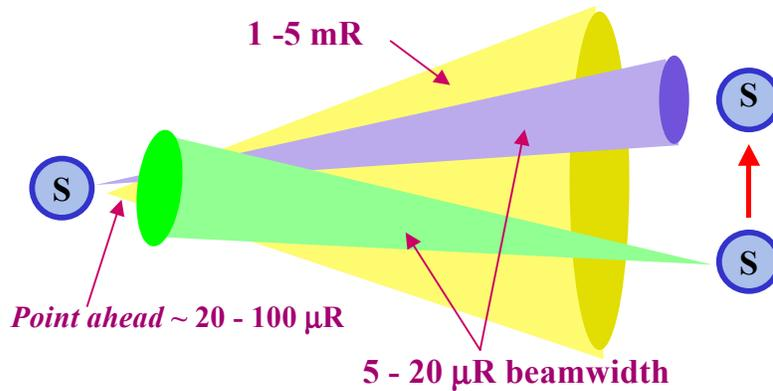
Figure 5. Spatial acquisition geometry.
