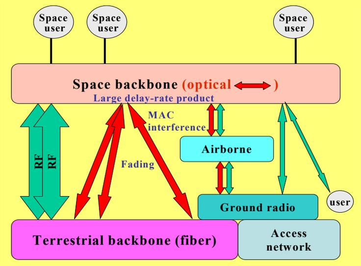
Figure 2. Logical network connection of different links in an integrated space-terrestrial network with major link properties that affect network performance and drives network architectures.
