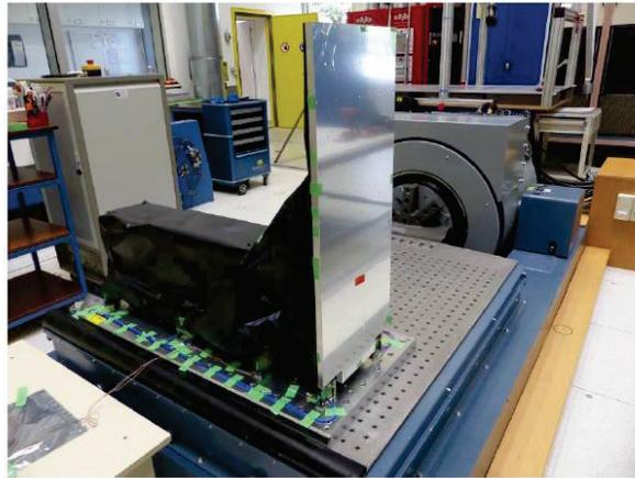
Figure 6. EEA engineering model – including MLI – on the shaker.
