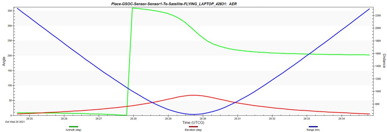
Figure 3. Az-El-Dist Plot of the specific downlink.
