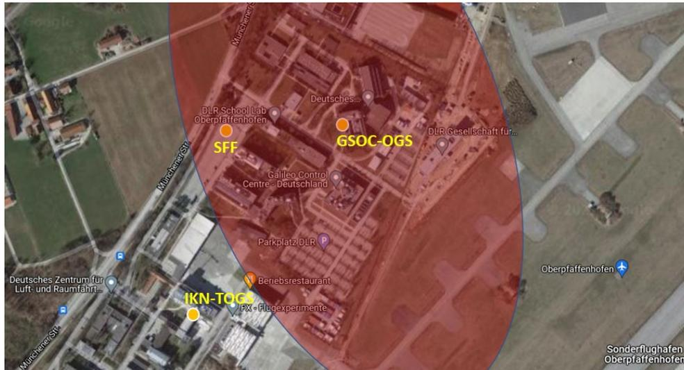
Figure 4. Aerial view of the receiver-site, indicating the locations of the three OGS. North is at top. The red area shows the ideal FWHM beam intensity at  $\sim 25^\circ$  link elevation, centered on the GSOC-OGS. The three OGS-locations approx. resemble a rectangular triangle, with leg distances of: GSOC-SFF  $\sim 172\text{m}$  and SFF-IKN  $\sim 290\text{m}$ .
