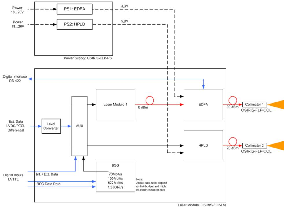
Figure 2. OSIRISv1 setup, as located onboard FLP.
