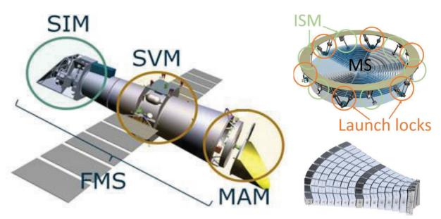
Figure 1: (Top left) Overview of the ATHENA spacecraft. (Top right) The MAM including the 2.6 m diameter aluminium alloy Mirror Structure (MS) with the 600 pockets where the MMs are placed, the launch locks and the Instrument Switching Mechanism (ISM). (Bottom right) Distribution of the SPO MMs along one of the sectors of the MAM.
