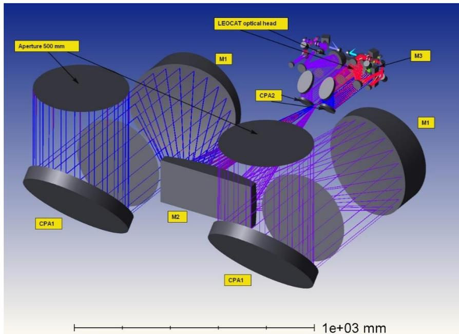
Figure 5. Proposed optical system layout of the QKD system in the space segment in isometric view. CPA: coarse pointing assembly, M: mirror. Colours of rays refer to transmission, receiving and tracking paths.
