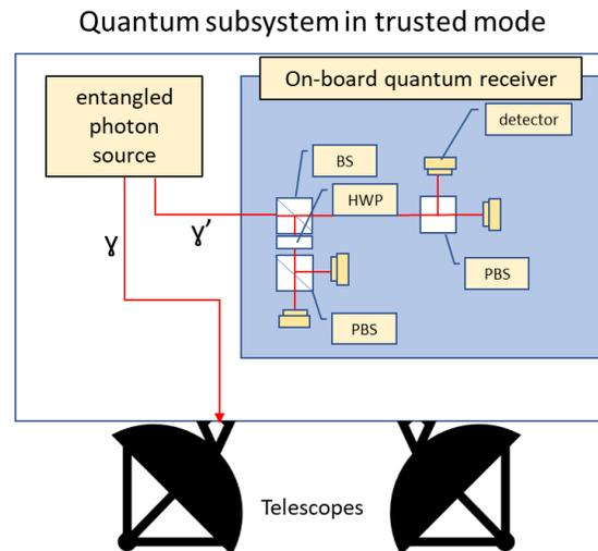
Figure 7. Sketch of the quantum subsystem in the space segment used for operation in trusted mode. BS=beam splitter, PBS=polarization beam splitter, HWP=half wave plate.
