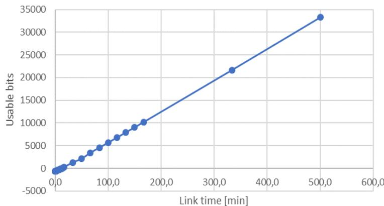
Figure 2. Simulated number of usable bits as a function of link time for the BBM92 protocol in untrusted mode, assuming a security parameter of  $10^{-12}$ , dark count of  $1000\text{Hz}$ , a source rate of  $10\text{GHz}$ ,  $2 \times 41\text{dB}$  link loss and an error correction efficiency of 1.22.
