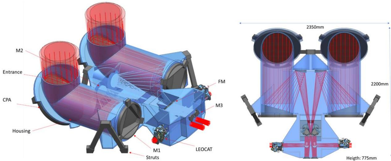
Figure 6. Mechanical design of the QKD payload in the space segment.
