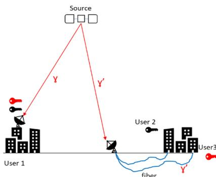
Figure 3. Sketch illustrating the two possible configurations of a free space and fibre coupling to detectors. Left: User 1 receives photons from the satellite containing the entangled photon source. These are directly measured near the telescope using a free-space link to the detectors. Right: photons are collected using a shared telescope, ideally outside an urban area; photons are coupled into an optical fibre leading the photons, via optical switches, to different users.
