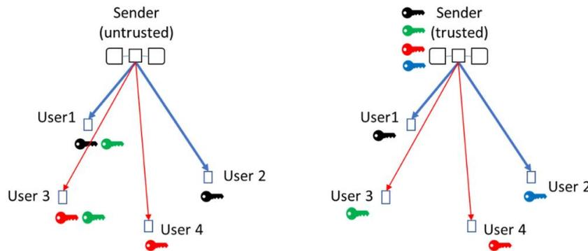
Figure 1. Two concepts studied in GEOQKD. Left: the satellite acts as an untrusted node, allowing to generate secure bits between different users on ground. Right: the satellite acts as a trusted node, creating keys between satellite and users on ground.
