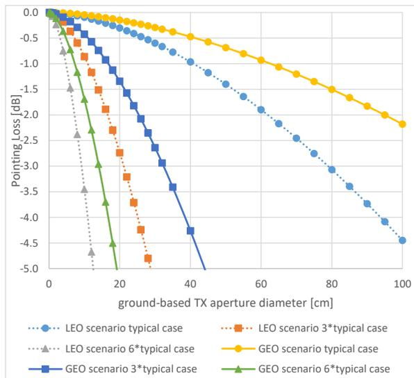
Figure 7. Pointing loss (in dB) as a function of the ground-based transmitter aperture diameter (in cm) due to residual differential tip-tilt. Solid lines (respectively dashed lines) correspond to GEO scenario (respectively LEO scenario). “Typical case” means one rms differential tip-tilt value is considered (values in Figure 6 b). Additionally, the curves for  $3^*$ rms and  $6^*$ rms values are depicted. The calculations assume a ground-based transmitter laser at 1064nm wavelength.
