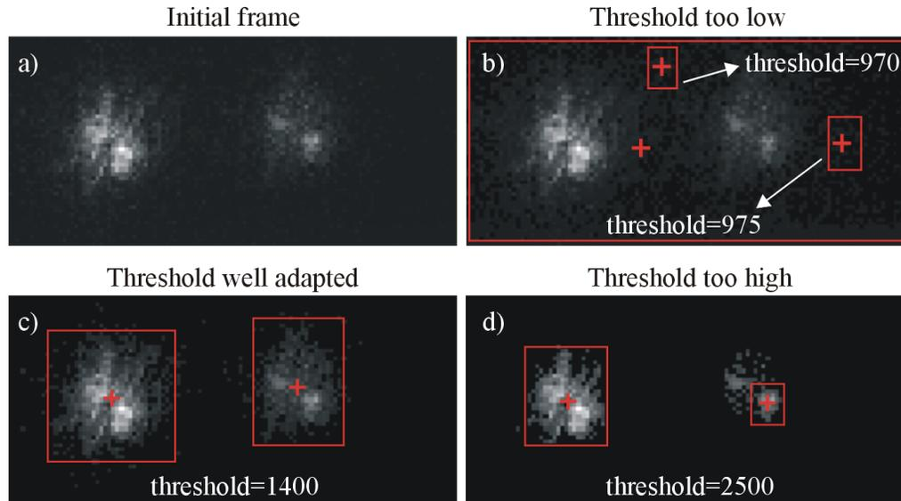
Figure 4: a) Initial frame; b) two different thresholds are applied: 970 and 975. The red rectangles show the four areas identified by the algorithm (one per star and per threshold). The largest rectangle is similar for both thresholds (the crosses are superimposed). If the threshold passes from 970 to 975, the algorithm gives a very different result; c) the algorithm converges, it identifies correctly the stars; d) the threshold is too high, one of the stars is over-segmented.
