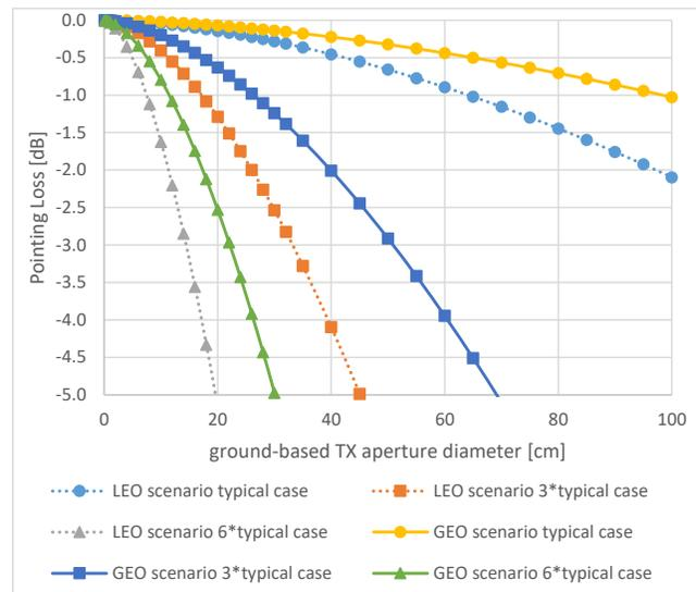
Figure 8. Pointing loss (in dB) as a function of the ground-based transmitter aperture diameter (in cm) due to residual differential tip-tilt. Solid lines (respectively dashed lines) correspond to GEO scenario (respectively LEO scenario). “Typical case” means one rms differential tip-tilt value is considered (values in Figure 6 b). Additionally, the curves for  $3^*$ rms and  $6^*$ rms values are included. The calculations assume a ground-based transmitter laser at 1550nm wavelength.
