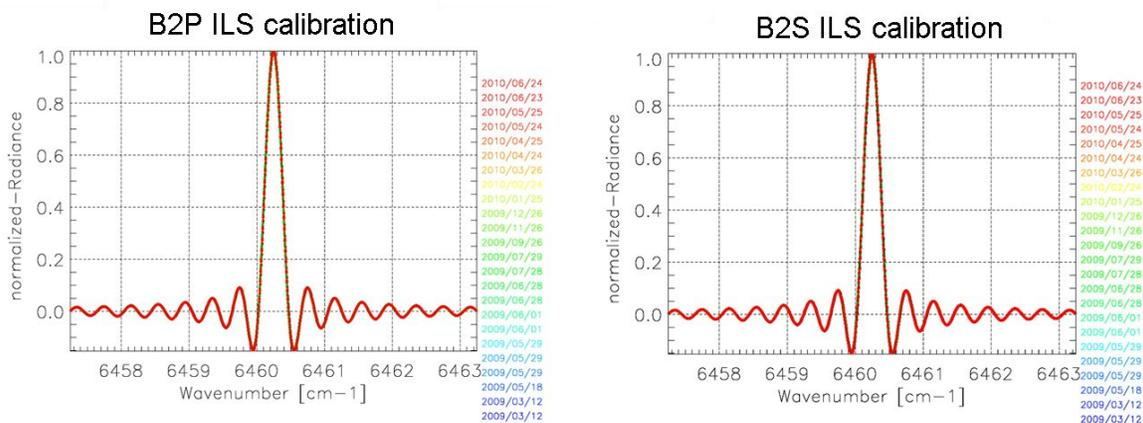
Fig. 5. ILS calibrations of Band 2 P and S by 1.55 micron on-board laser in one year
