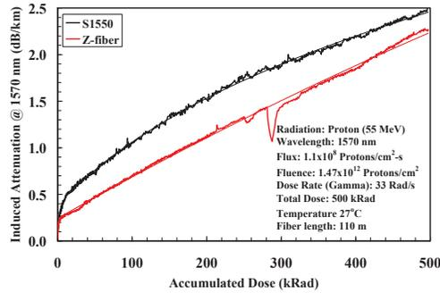
Fig. 6. Proton radiation data of S1550-HTA and Z-fiber®.
