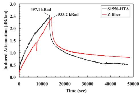
Fig. 5. Proton test data of S1550-HTA fiber.
