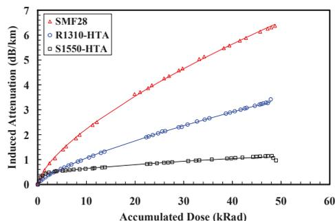
Fig. 1.  $\gamma$ -radiation data of the SM fibers.
