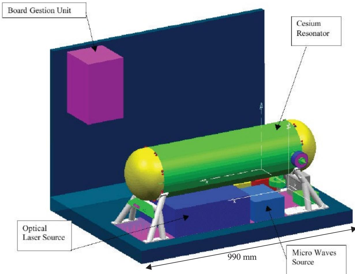
Figure 1 - 3D view of the PHARAO instrument
