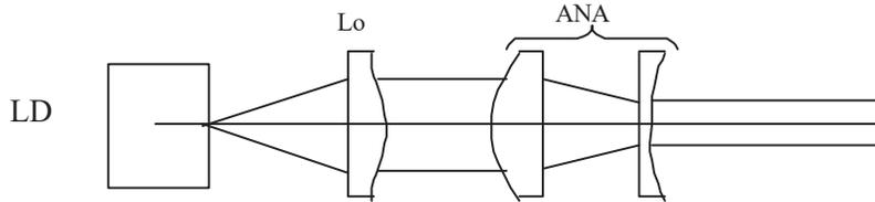
Figure 5 - Source Laser Diode and its anamorphoser
