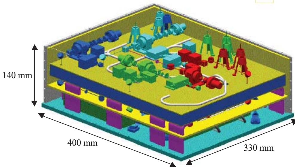
**Figure 3 - 3D view of the Laser Source subsystem**
