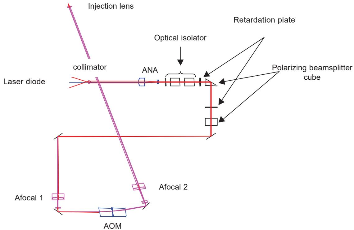
Figure 7 - Global view of the capture beam generation system
