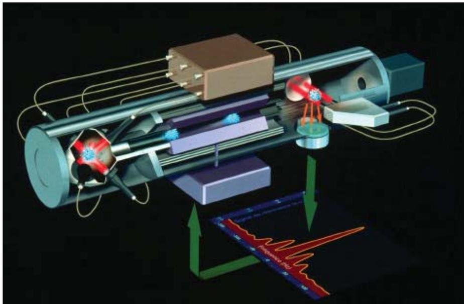
Figure 2– Atomic clock principle in microgravity
