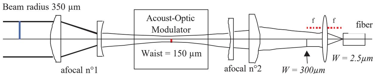
Figure 6 - The acousto-optic modulator and its optics
