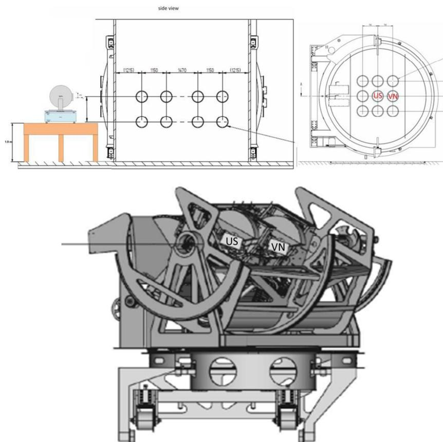
**Fig. 2.** Instrument mounted in the TRS in CAS measurement configuration (US and VN sun baffles indicated) as viewed from the OGSE. Note the independent rail supports for the instrument and CRAS. (credits APCO/RAL)
