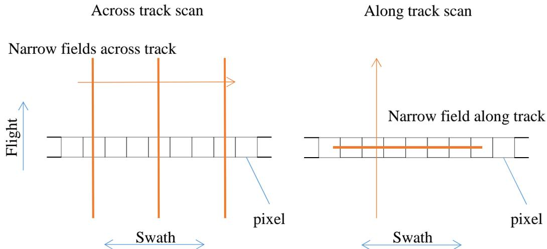
Fig. 5. Field of view scan principle.
