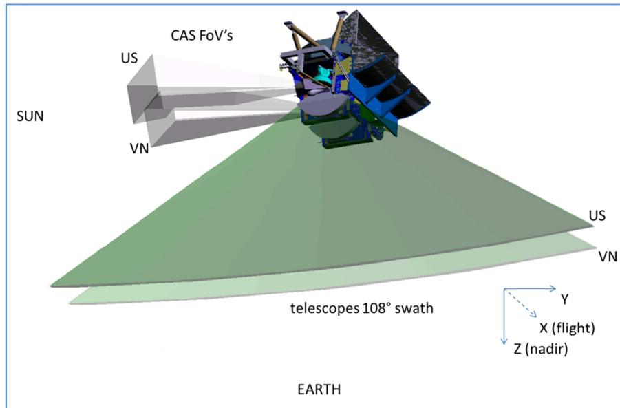
**Fig. 1.** Sentinel-5 instrument configuration showing the telescopes FoV towards Earth and the Calibration subsystem FoV towards the sun over the South Pole.
