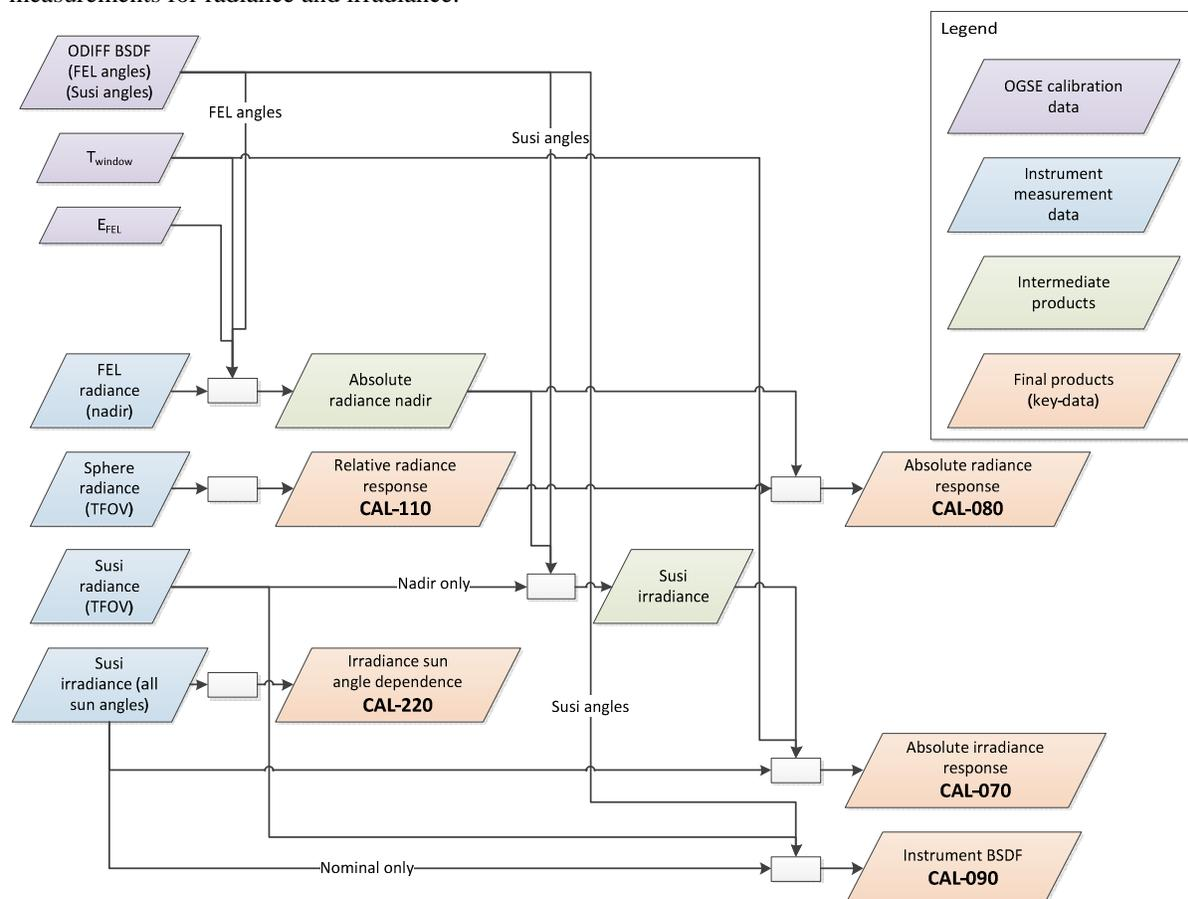
Fig. 4. Determination of the radiometric key-data from measurement data.
