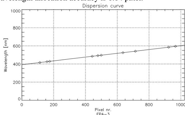
**Fig. 3.** Dispersion curve determined for the FPA-3 of the GOME-2 instrument. The diamonds indicate the spectral emission lines of the source used as fitting points.
