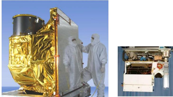
Figure 6. A comparison of the GOES ABI (left) and the S-NPP CrIS sensor (right) size. ABI's optical aperture diameter is almost 10 times that of the 8 cm aperture on CrIS.
