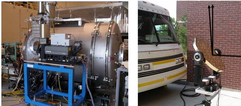
Figure 9. (Left) The GIFTS thermal vacuum chamber with the window to allow viewing the outside environment. The UW AERI is located on the table near the chamber to provide a comparison measurement for the GIFTS data. (Right) Both systems view a large turning mirror outside the building to make vertical profile measurements.
