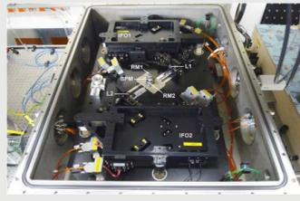
Fig 2: Measurement setup in the vacuum chamber.
