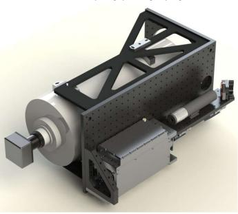
The Imaging Lidar consists of the UV laser and beam-expander in the foreground, with the 20 cm diameter (Meade) receiving telescope in the background. The "black box" at lower left is the Photek PCS-256 – the 32 \*32 Imaging Photon Detector (currently used with 16 \* 16 electronics).
