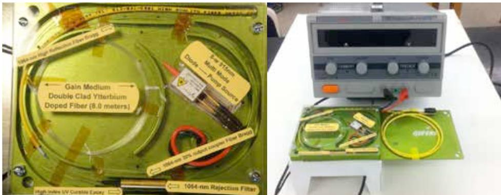
Figure 3 –(Right) Fiber laser gain medium and pump lasers (Left) Ytterbium-doped fiber laser demonstration unit.
