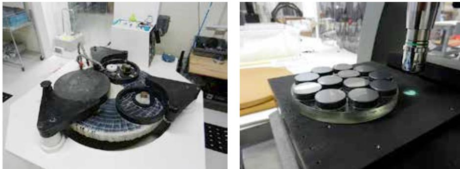
Figure 7- (Left) Roughness masters polishing on a 36 inch planetary polishing machine. (Right) Masters readied for measuring on a NewView white light scanning profilometer.
