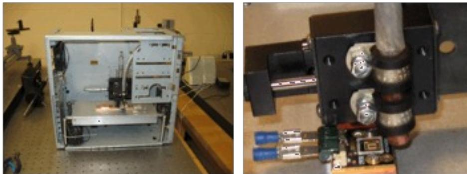
Figure 1 – (Left) Prototype LED enclosure. (Right) High powered LED mounted for x-y positioning.
