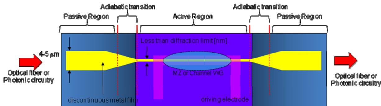
Figure 9. An EO modulator effecting sub-wavelength ( $\lambda$ ) concentration of light
