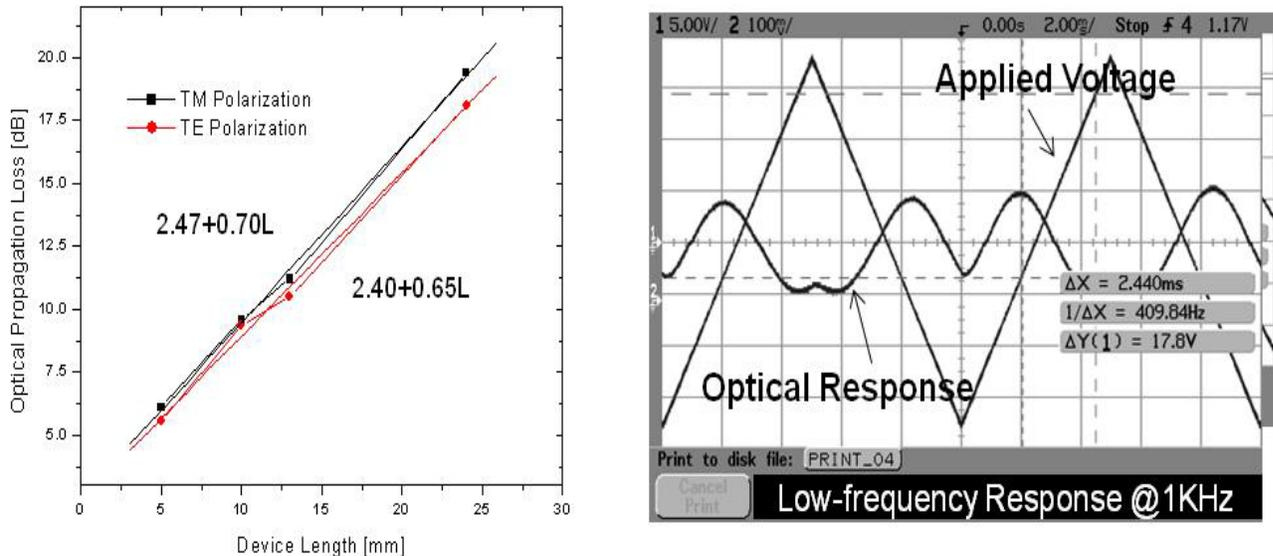
Figure 8. The optical loss (left) and electro-optic response (right) are shown for an IMI plasmonic structure prepared using the DH6-APC OEO material.
