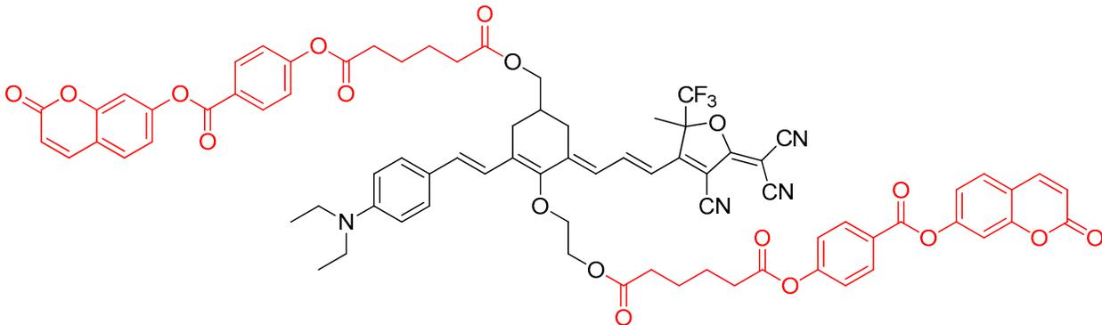
Figure 5. The structure of a new EO material currently being synthesized is shown. Variants, where the coumarin moieties are attached to the ends of the chromophore, are also being prepared.
