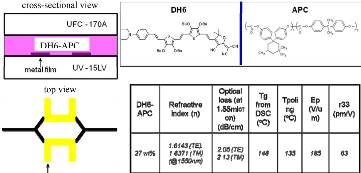
Fig. 7. Cross-sectional and top views of the push-pull Mach Zehnder amplitude modulator employing discontinuous (nanostructured) metal films are shown as is the structure of the DH6 chromophore and the host APC polymer. Also shown are the characteristics of the DH6-APC composite and the poling condition.
