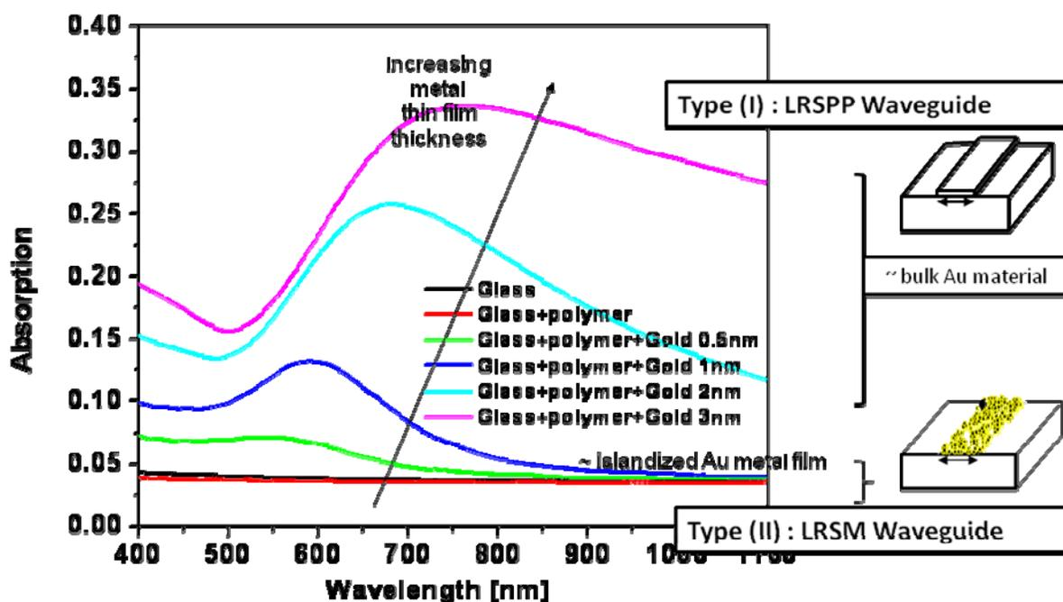
Figure 6. Absorption of spectra as a function of discontinuous gold film thickness and illustration of the transition from LRSM to LRSP behavior.
