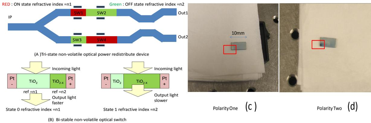
Fig.7 transition metal oxide based switch (a),(b) MZI based tri-state switch, (c)(d) non-volatile change of optical property.
