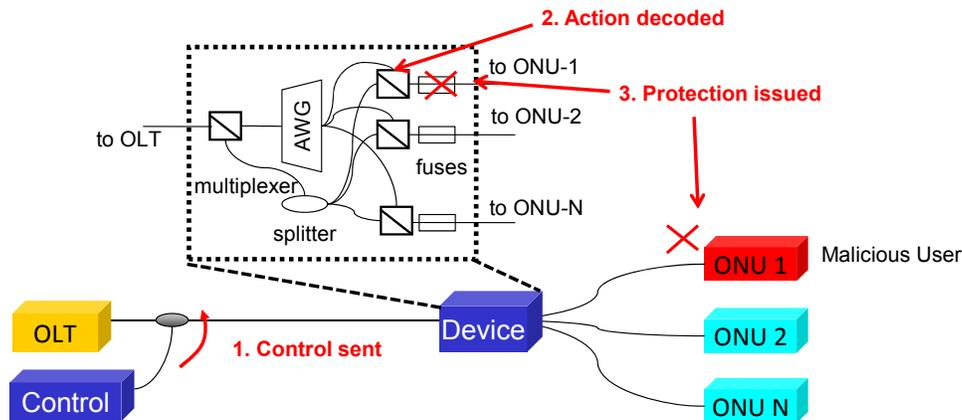
Fig.4 Node architecture of optical countermeasure
