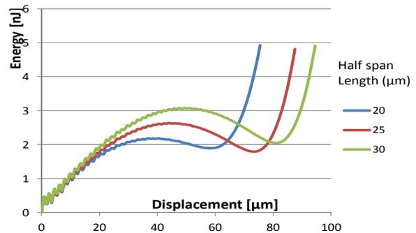
Fig.6b latching property of tri-state MEMs
