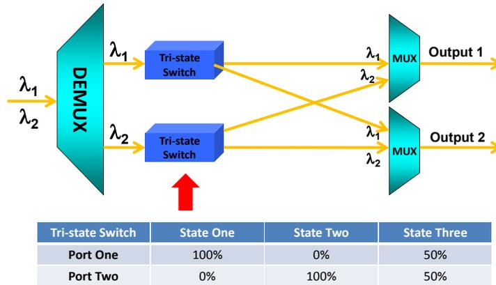
Fig.5 Tri-state example for reconfigurable router
