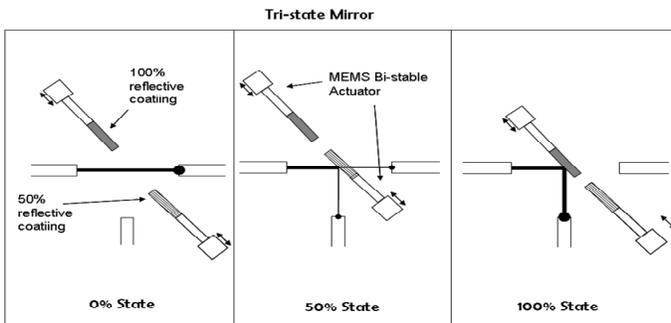
Fig.6a Tri-state MEMs
