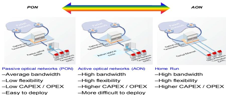
Fig.1 Optical Access Network Technology
