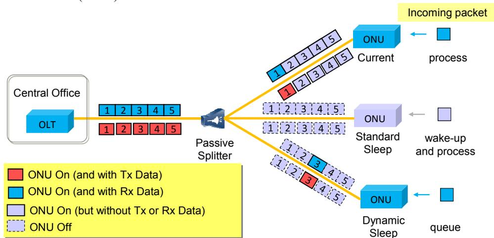
Fig.8 Energy saving using dynamic sleep mode
