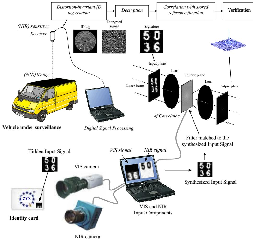
Fig. 7. ID tag readout, signature decryption and comparison with the input signal in an optical correlator for verification.
