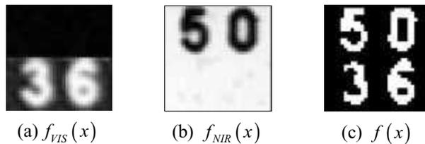
Fig. 1. Example 1: (a) VIS and (b) NIR images of the reference signature. (c) Synthesized signature after applying Eq. (1).
