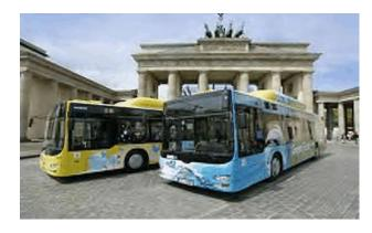
Figure 8. Two Hydrogen Internal Combustion Engine Buses in Berlin, Germany
