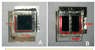
Picture A: a single with a 1cm-by-1cm size (η =7.5% Jsc=20.1mA/ cm2, Voc=0.68V, ff=0.59)
