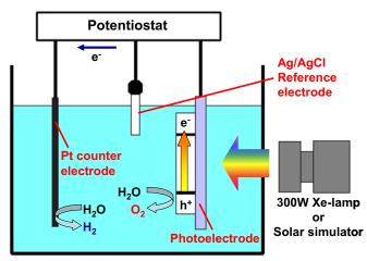
Fig. 3. Photoelectrochemical cell set up
