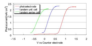
Fig. 9 Three I-V curves of WO<sub>3</sub> photoelectrode systems under simulated solar light irradiation (AM1.5, 100mW/cm<sup>2</sup> one sun).
