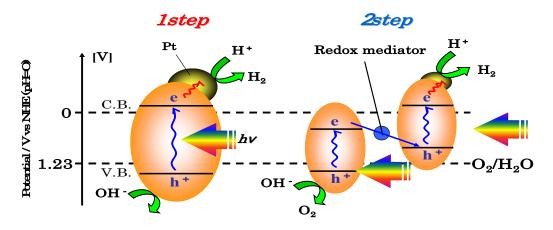
Fig. 1. Water splitting mechanisms using powder photocatalysts of metal promoted oxide semiconductor
