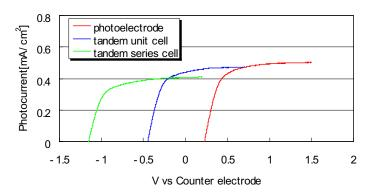
Fig. 8 Three I-V curves of TiO<sub>2</sub> photoelectrode systems under simulated solar light irradiation (AM1.5, 100mW/cm<sup>2</sup>, one sun).
