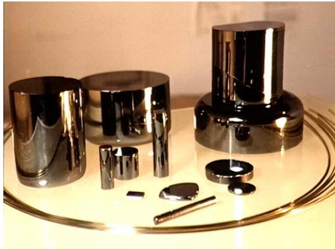
Figure 2 : Bulks of selenide glasses in various sizes photographed with optical fibers.
