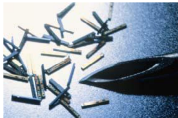
Figure 4. Pressure sensor chips beside a cannula needle.
