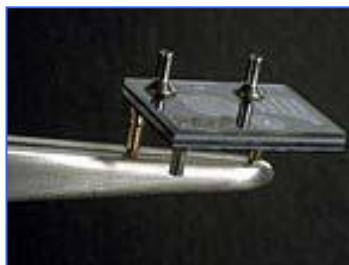
Figure 2. Micropump for drug delivery applications.
