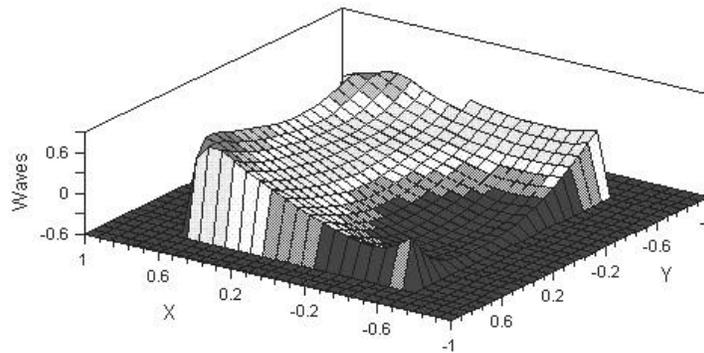
Figure 3. The corrected field of a high resolution c-mount lens, with less than 0.1 percent distortion.
