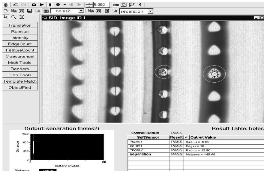
Figure 5. Typical smart camera applications of edge measurements and feature counting.
