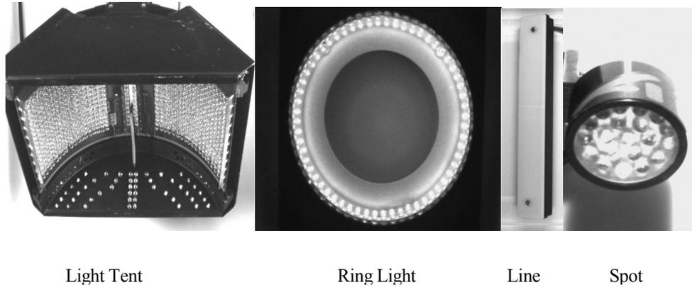
Figure 2. Some new lights showing flexibility of design using LEDs
