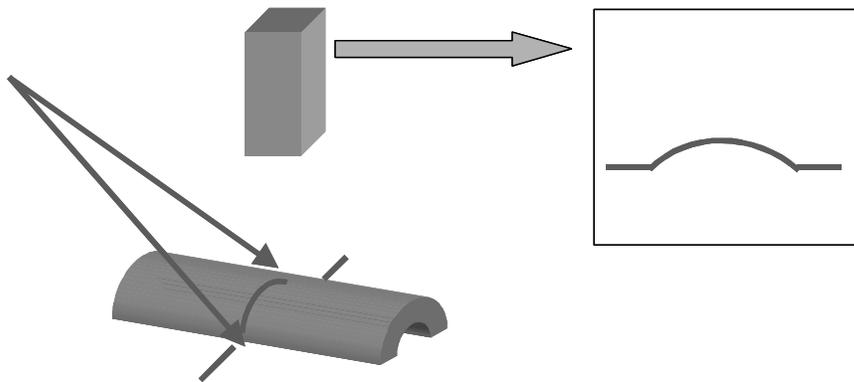
Figure 6. Basic laser triangulation system using lines of light.
