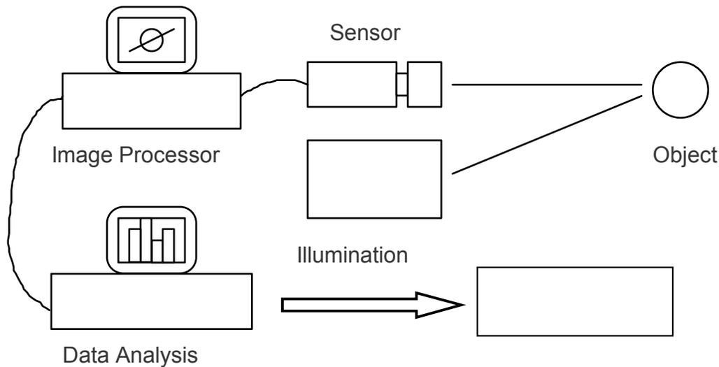
Figure 1. Block Diagram of a typical Machine Vision System.
