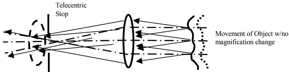
Figure 4. A telecentric optical system collects a constant perspective, magnification and cone of light across the part.
