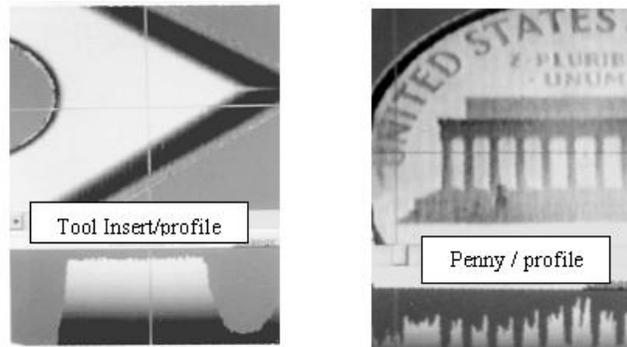
Figure 7. Examples of 3D gray scale depth maps, where the Z depth dimension is represented by grey level.
