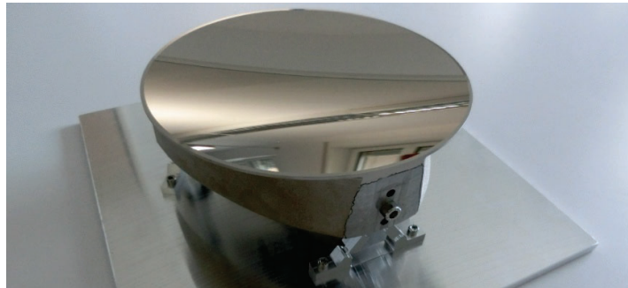
Figure 2 AM mirror demonstrator developed and manufactured within previous ESA GSTP.
