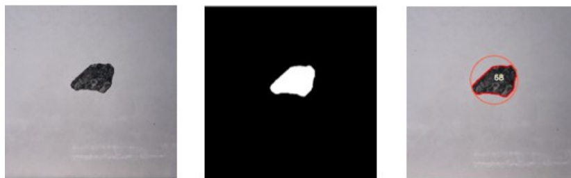
Figure 7. Image segmentation results and particle size calculation.
